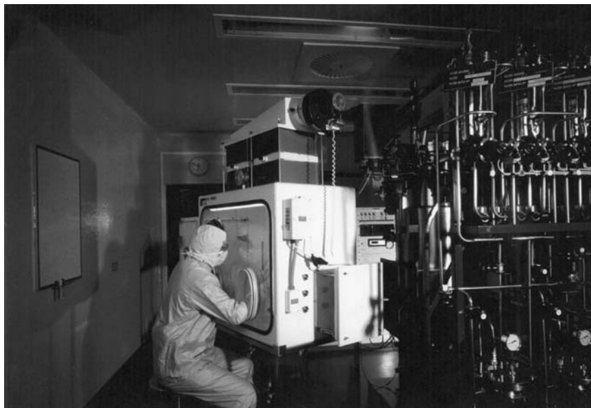
Figure 3.1 Class III microbiological safety cabinet. The safe manufacture of botulinum toxins requires containment of various unit processes in cabinets of this type that operate under negative pressure and provide a secure physical barrier between the product and the operator.
