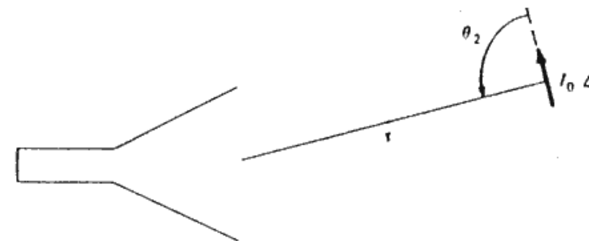
Figure 5.3 Orientation of current element for maximum received power.
