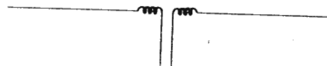
Figure 3.6 Short dipole antenna with tuning coils at the input.
